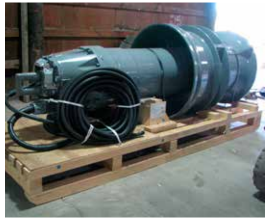
Flygt PL-7101/300-hp explosion-proof electric submersible propeller pump unit awaiting installation.
